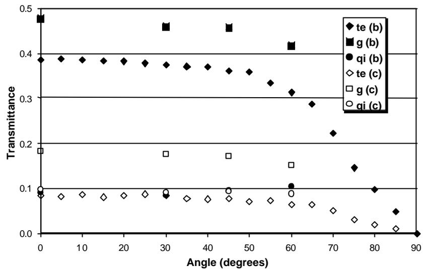
Fig. 2: Angle dependent energy transmittance of a triple glazed gasochromic IGU ( $t_e$  solar transmittance;  $g$  total solar energy transmittance;  $q_i$  secondary heat gain factor; (b) bleached state; (c) coloured state (Source: Fraunhofer ISE report to SWIFT, cited in [10]).
