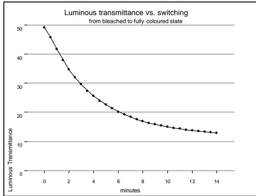
Fig. 1.: Rate of change in the visible transmittance for an electrochromic double glazed unit as specified in Table 2 [7].
