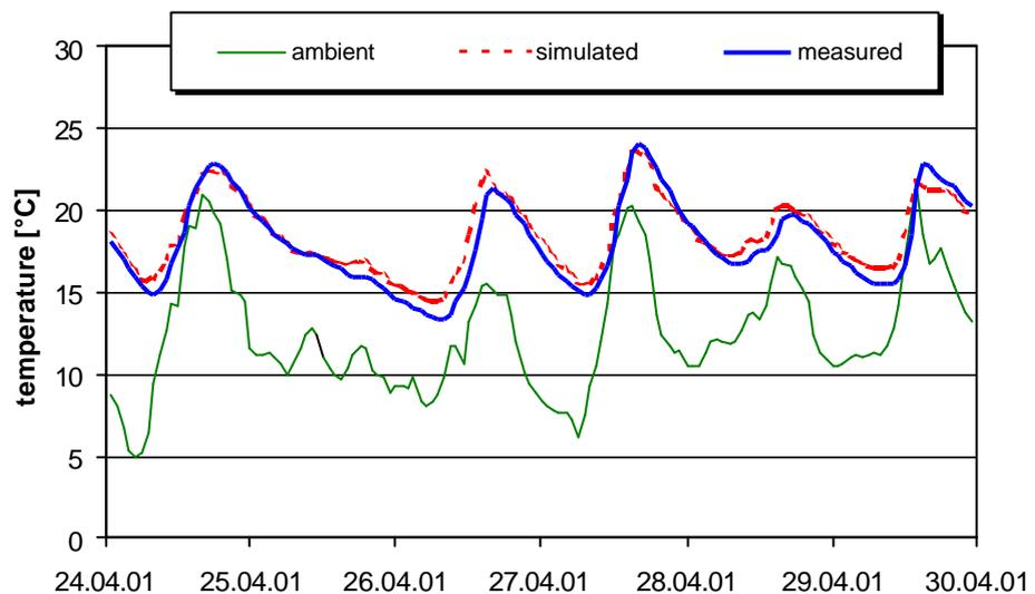
Fig. 3: Comparison of measured and simulated air temperatures in the FASTEST test cabin equipped with gasochromic glazing (Source: Fraunhofer ISE report to SWIFT).
