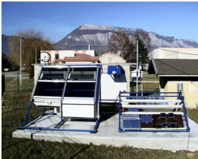
Fig. 7: Outdoor test stand for chromogenic glazing and meteorological measurements at CSTB, Grenoble. (Source: CSTB report to SWIFT).
