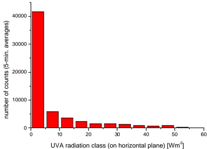
Fig. 5: Frequency distribution of UVA radiation on horizontal plane, measured at Freiburg, Germany. 5-minute averages, December 2001 to June 2002. (Source of data: Fraunhofer ISE).
