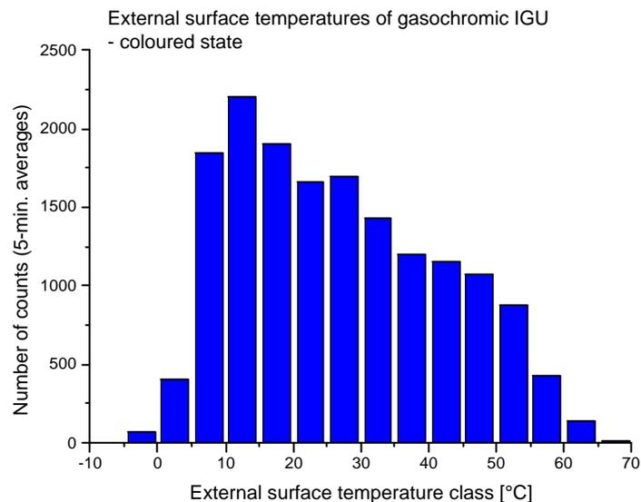
Fig. 4: Distribution of the external glazing surface temperatures for gasochromic triple glazed units in the coloured state, tilted 45° and orientated south for outdoor exposure tests at Freiburg, Germany. 5-minute averages, December 2001 to June 2002. (Source of data: Fraunhofer ISE).
