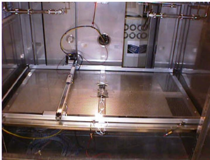
Fig. 6: Sample exposure plane inside the accelerated weathering unit at NREL for accelerated testing of electrochromic windows according to [18] (Source: NREL).
