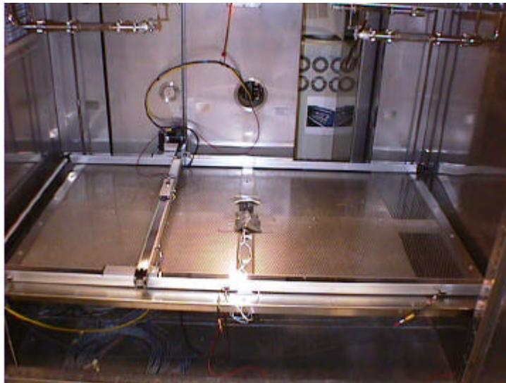
Fig. 6: Sample exposure plane inside the accelerated weathering unit at NREL for accelerated testing of electrochromic windows according to [18] (Source: NREL).
