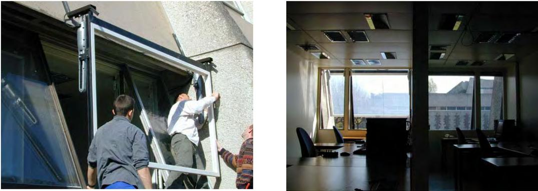
Fig. 4-13: Real 1:1 scale experiment within the TwinCells (right). Left Room is equipped with tiltable Serraglaze window (left).
