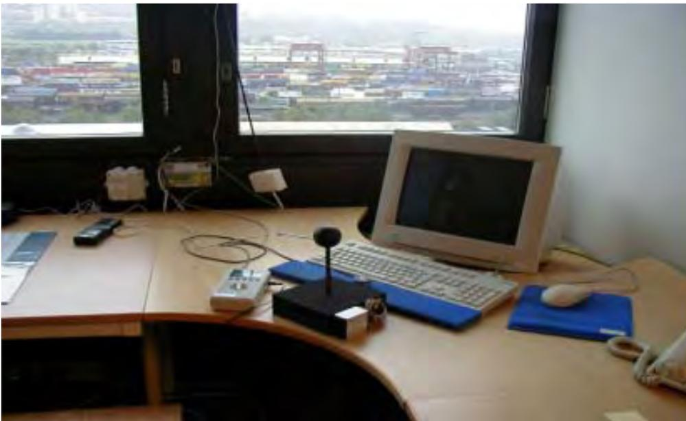
Figure 18: South facing office at SIEMENS Linderud. Measurement of operative temperature.
