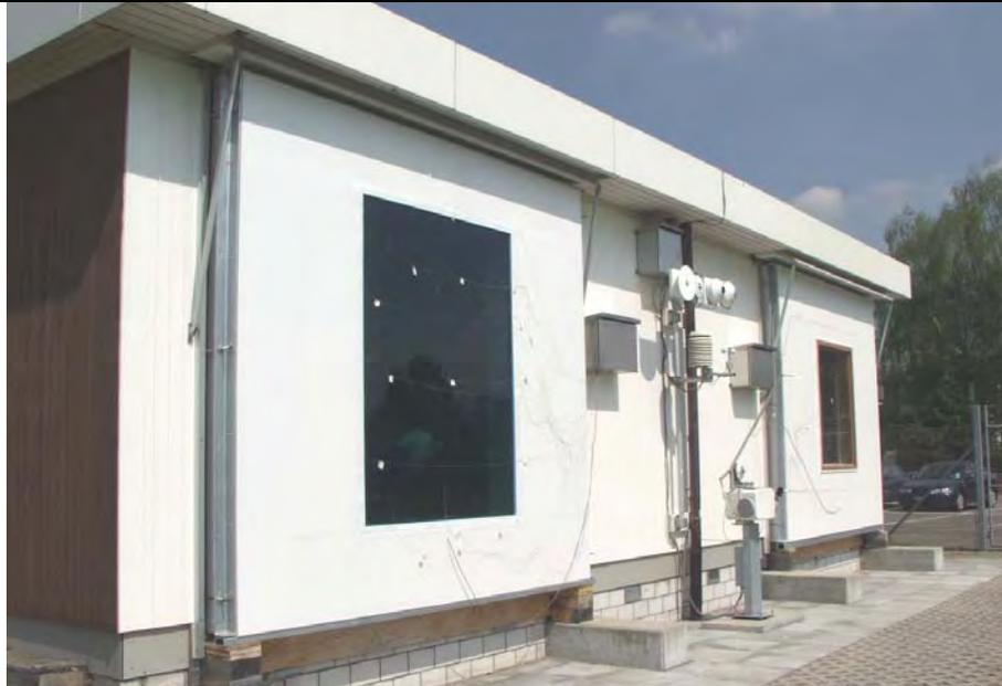
Figure 1-3: EMPA outdoor test facility. Two test cells are built in a wooden building. Temperature controlled indoor air is flowing around the cell walls except for the test face which is exposed to the environment. Climate data sensors including a tracker for direct normal radiation are located between the two test faces.
