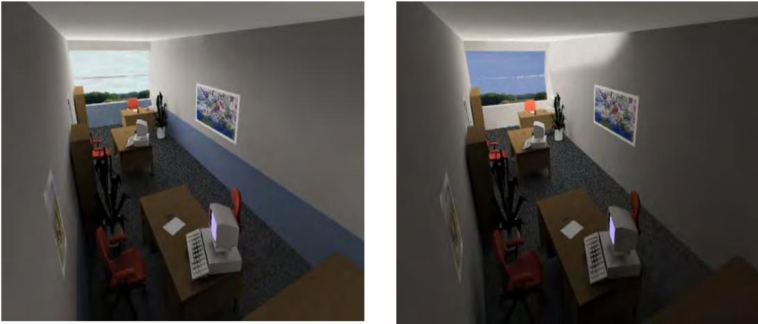
Fig. 11: Daylighting simulation of simple glazing (left) and Serraglaze (right) – Opposite views.
