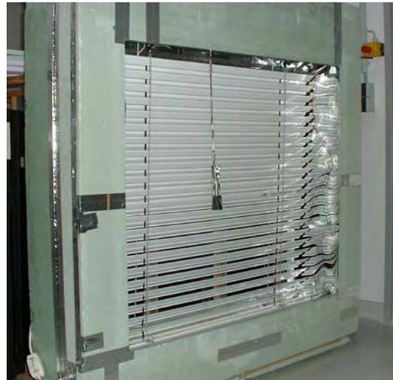
Figure 1-2: Solar calorimeter (ISE) with mounted exterior Venetian blind (left). Test frame for interior Venetian blinds (right).
