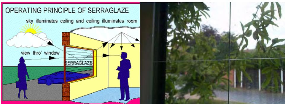
Fig. 4-4: Operating principle of the Serraglaze product (left), and view through the window (right).
