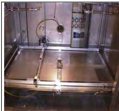
Fig.4: Interior view of the climatic chamber at NREL, showing the scanning radiometer for homogeneity measurements.
