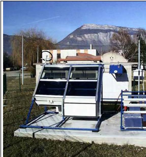
Fig. 6: View of the test box for outdoor exposure and meteorological instruments at CSTB
