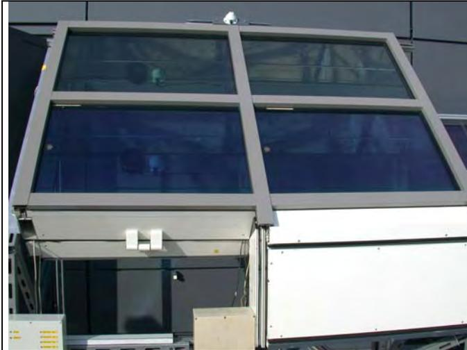
Fig. 7: View of the test box for outdoor exposure in Freiburg (back absorber plate removed for better visibility).
