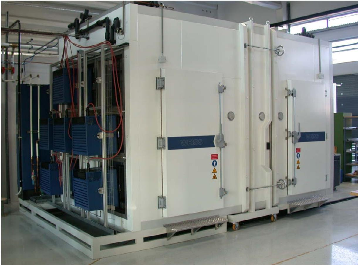
Fig.3: Double climatic chamber at Fraunhofer ISE.
