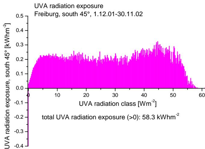
Fig. 3: Global UVA radiation distribution on a 45°-tilted, south-oriented plane in Freiburg, 1.12.01-30.11.02
