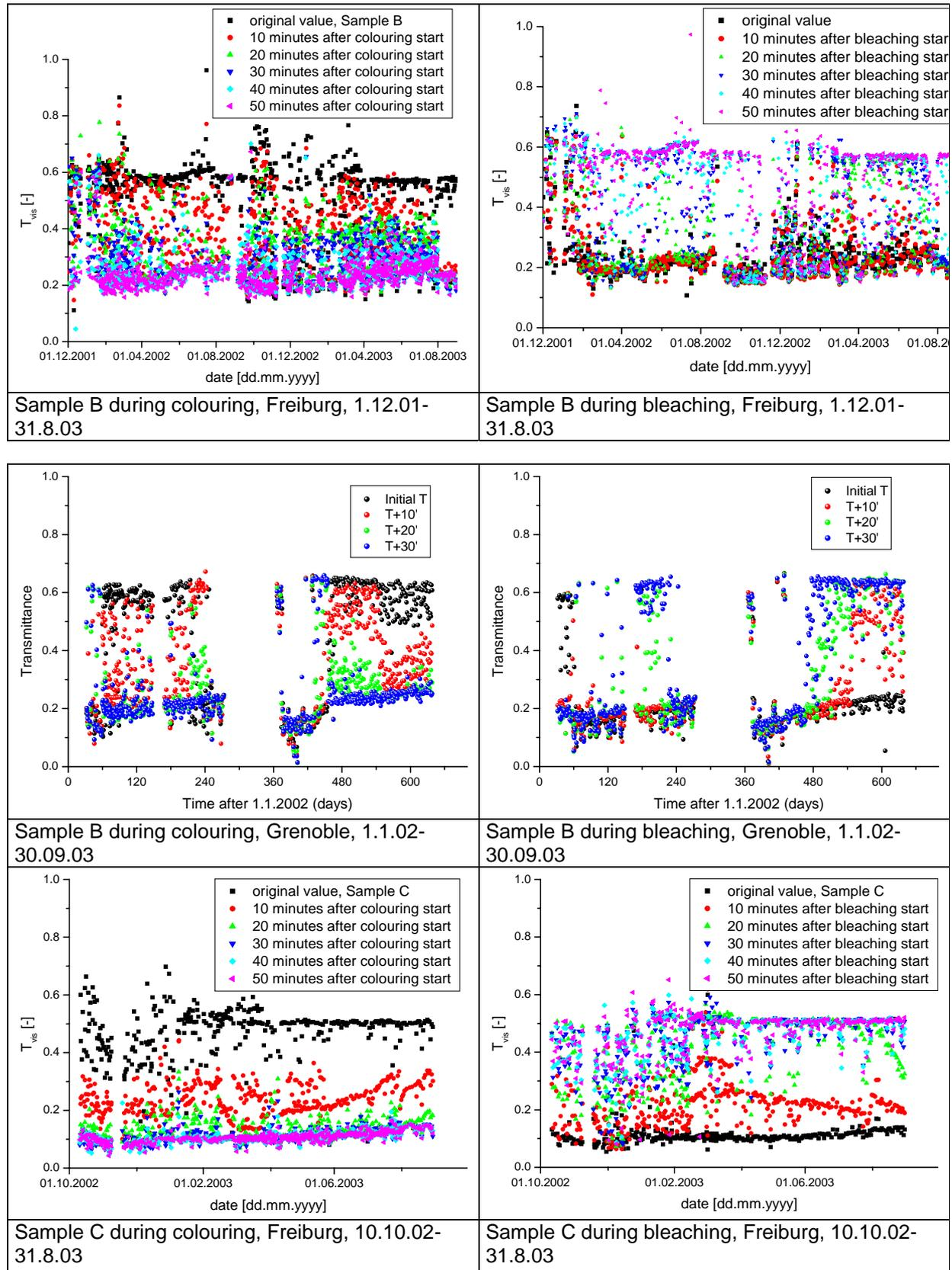
Fig. 13: Transmittance values at 10-minute intervals after the beginning of colouring or bleaching for the chromogenic glazing samples A, B and C, exposed outdoors in Freiburg and Grenoble
