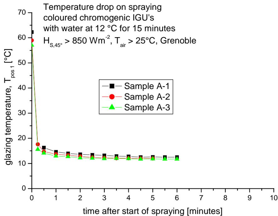
Fig. 12: Glazing surface temperatures during the thermal shock test (Table 1, SWIFT 5) in Grenoble
