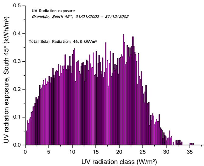
Fig. 7: Global UVA radiation distribution on a 45°-tilted, south-oriented plane in Grenoble, 1.1.02-31.12.02
