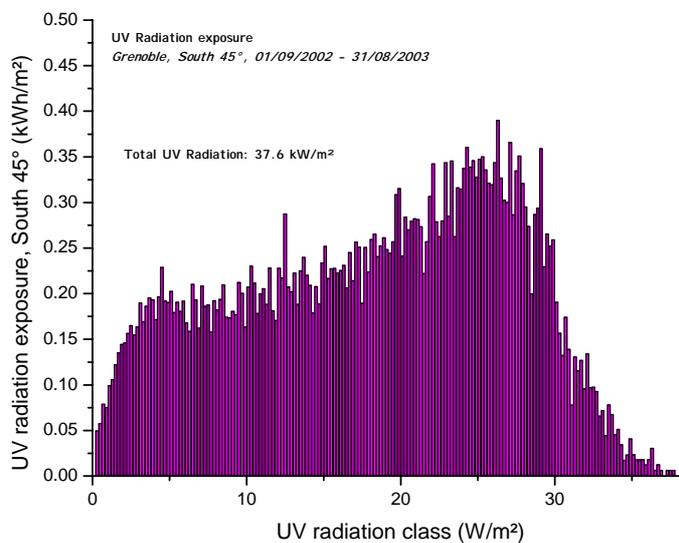
Fig. 8: Global UVA radiation distribution on a 45°-tilted, south-oriented plane in Grenoble, 1.9.02-31.8.03
