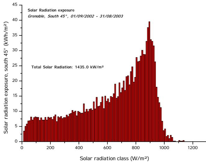
Fig. 6: Global solar radiation distribution on a 45°-tilted, south-oriented plane in Grenoble, 1.9.02-31.8.03
