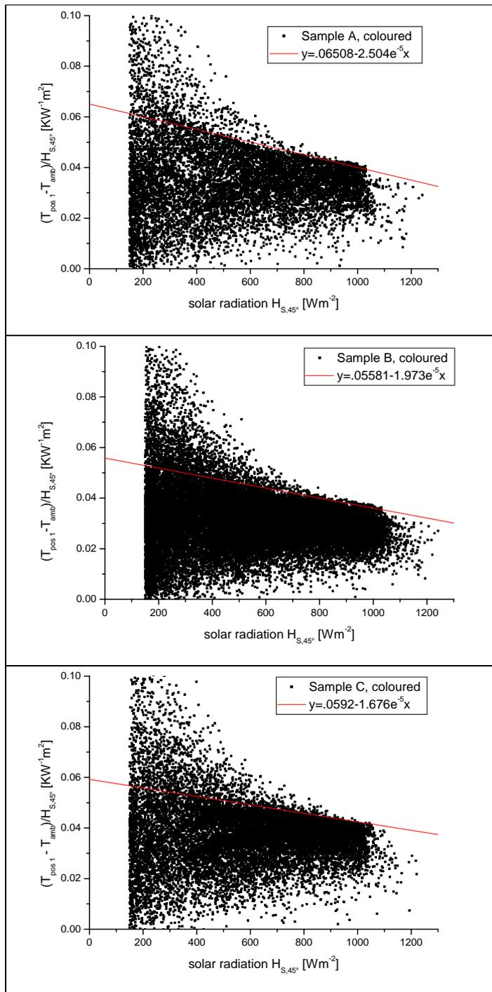
Fig. 10: Radiation-scaled temperature difference between glazing surface and air temperatures, versus global solar radiation in the glazing plane, for the three chromogenic glazing systems in the coloured state, exposed in Freiburg.
