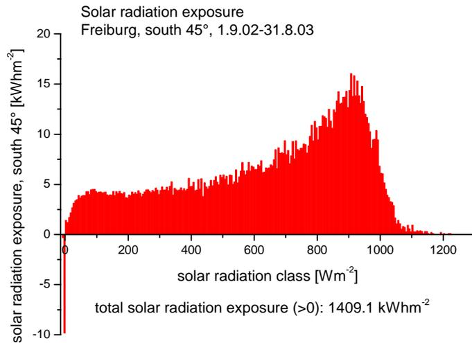
Fig. 2: Global solar radiation distribution on a 45°-tilted, south-oriented plane in Freiburg, 1.9.02-31.8.03
