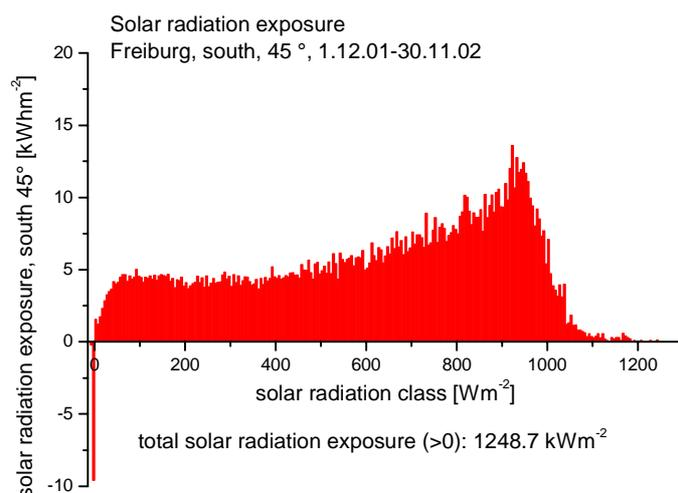
Fig. 1: Global solar radiation distribution on a 45°-tilted, south-oriented plane in Freiburg, 1.12.01-30.11.02
