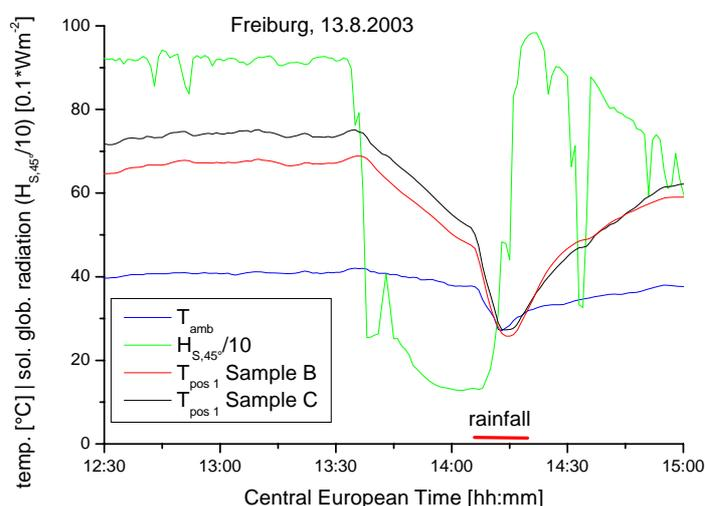
Fig. 11: Meteorological data and glazing surface temperatures during a summer thunderstorm in Freiburg
