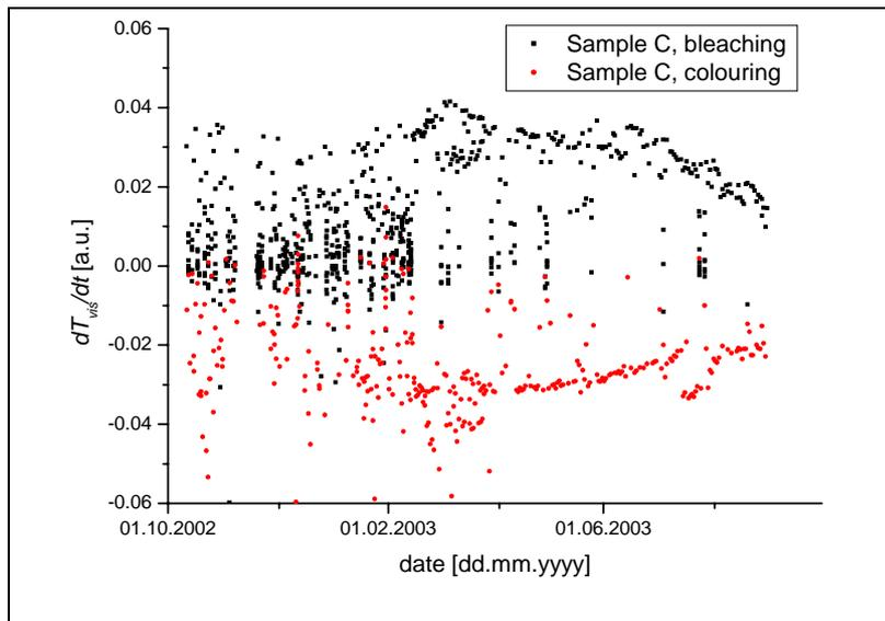
Fig. 14: Change over time of switching rates (black - bleaching; red - colouring) in arbitrary but identical units for samples A, B and C, exposed outdoors in Freiburg.
