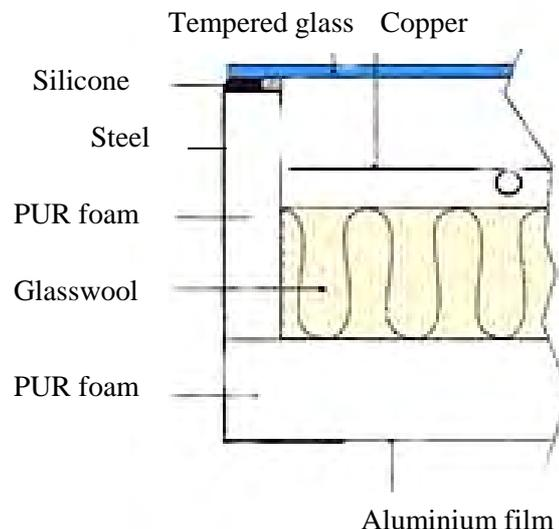
Functional Unit : It is a solar collector with an optical factor  $B=0,72$  and a transmission coefficient  $K=4,36 \text{ W/m}^2\cdot\text{K}$  which produce energy during 10 years.
