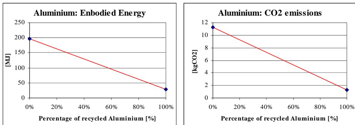
**Fig. 3: Embodied energy and CO<sub>2</sub> emissions for variable percentages of recycled aluminium in the aluminium sheet**
