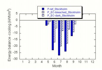
Fig. 6: Energy balance for cooling for a south facing window in Stockholm. The energy balance is given in kWh per square metre of window area.
