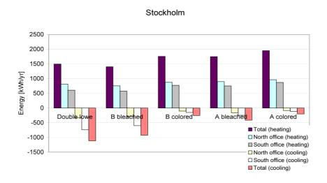
Fig. 4: Heating and cooling loads for the north and south office modules equipped with two of the switchable windows (A and B) and the reference window (double low-e) in Stockholm
