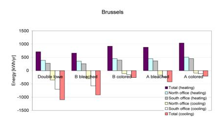
Fig 3: Heating and cooling loads for the north and south office modules equipped with two of the switchable windows (A and B) and the reference window (double low-e) in Brussels
