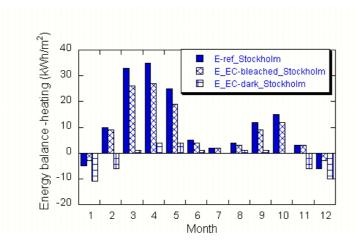
Fig. 5: Energy balance for heating for a south facing window in Stockholm. The energy balance is given in kWh per square metre of window area.
