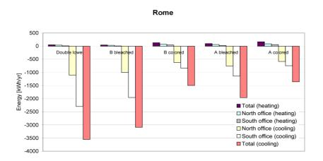
Fig 2: Heating and cooling loads for the north and south office modules equipped with two of the switchable windows (A and B) and the reference window (double low-e) in Rome
