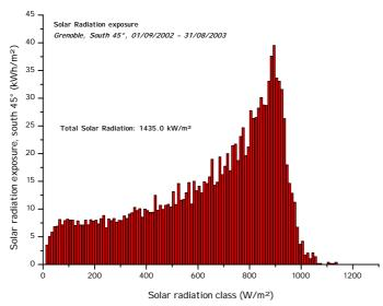
Fig. 6: Global solar radiation distribution on a 45°-tilted, south-oriented plane in Grenoble, 1.9.02-31.8.03
