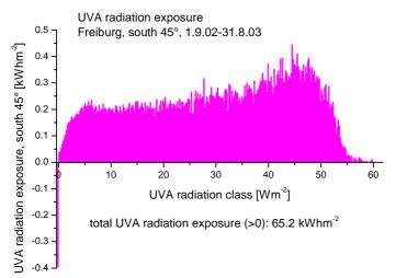
Fig. 4. Global UVA radiation distribution on a 45°-tilted, south-oriented plane in Freiburg, 1.9.02-31.8.03
