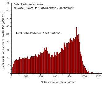
Fig. 5: Global solar radiation distribution on a 45°-tilted, south-oriented plane in Grenoble, 1.1.02-31.12.02
