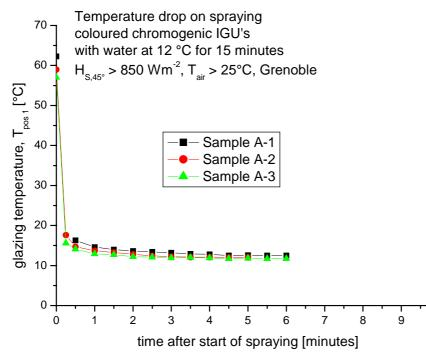
Fig. 12: Glazing surface temperatures during the thermal shock test (Table 1, SWIFT 5) in Grenoble
