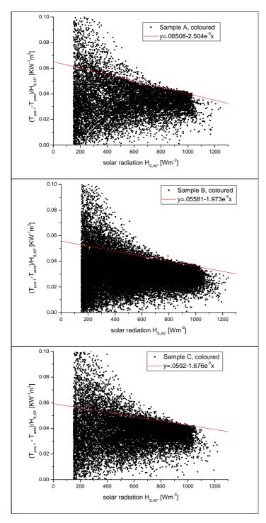
Fig. 10: Radiation-scaled temperature difference between glazing surface and air temperatures, versus global solar radiation in the glazing plane, for the three chromogenic glazing systems in the coloured state, exposed in Freiburg.
