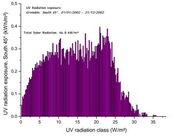
Fig. 7: Global UVA radiation distribution on a 45°-tilted, south-oriented plane in Grenoble, 1.1.02-31.12.02
