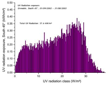
Fig. 8: Global UVA radiation distribution on a 45°-tilted, south-oriented plane in Grenoble, 1.9.02-31.8.03
